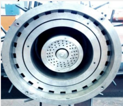
B 公司产品采用矩形可调结构, 调节所需扭矩大, 一次风抗干扰能力差, 燃烧器推力损失大 Burner nozzle from Company B: Adopts rectangular adjustable structure, which requires large torque for adjustment, poor in anti-interference of primary air, big loss for thrust of burner
