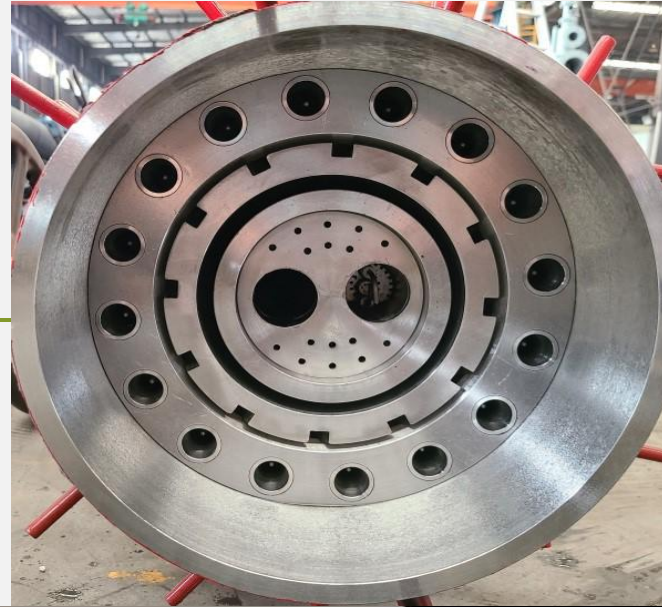
炬烽热能AVLS专利燃烧器, 拉瓦尔收敛扩散可调喷嘴, 调节所需扭矩小, 兼具可调性能和抗干扰能力 Generalflame AVLS patent burner: Laval convergent diffusion adjustable nozzle, low torque required for adjustment, Strong for adjustability and anti-interference ability
