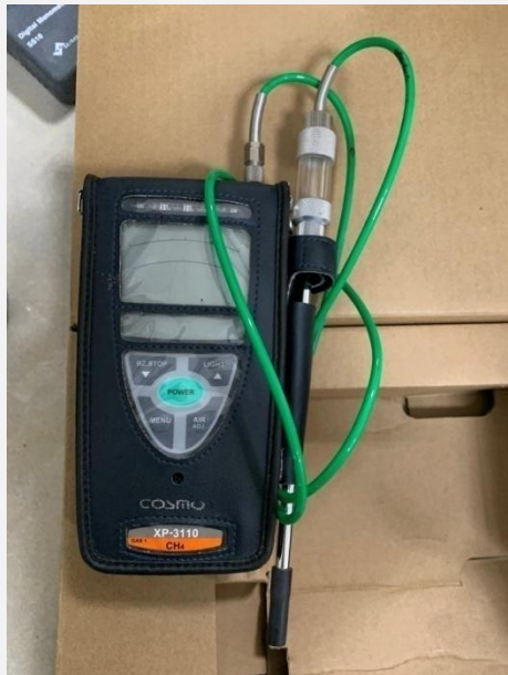
燃气泄露检测 Gas leakage test
