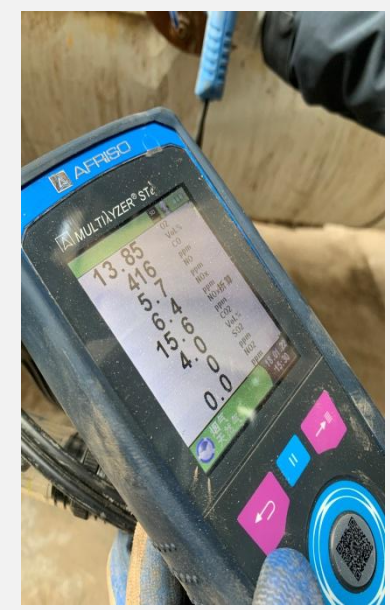
烟气检测 Flue gas test
